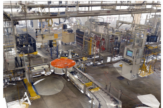
3D Point cloud model of a Ford motor car plant in the USA. Point cloud is comprised of ~4.5 billion points and is visualized using Pointools Edit.
