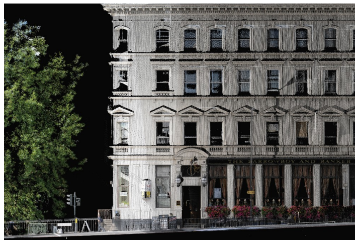
3D Point cloud model in AutoCAD, displayed using Pointools Plug-in for AutoCAD
